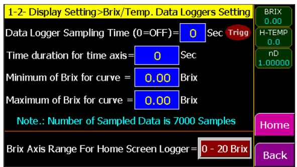
**Figure 6-3** Data Logger Setting
