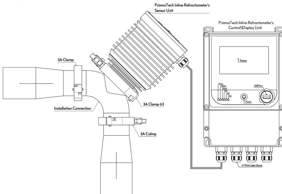
Figure 2-3 Refractometer Sensor Mounting
