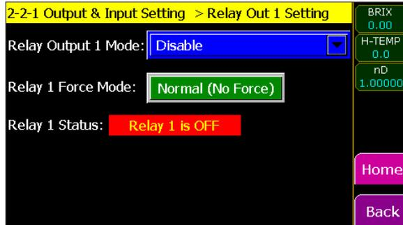
Figure 6-6 Relay Outputs Configuration page
