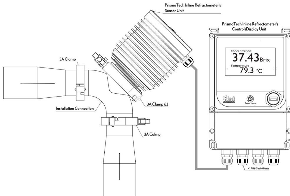
**Figure 1-1** Refractometer Equipment
