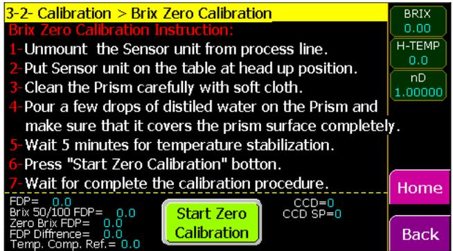
**Figure 6-9** Brix Zero Calibration
