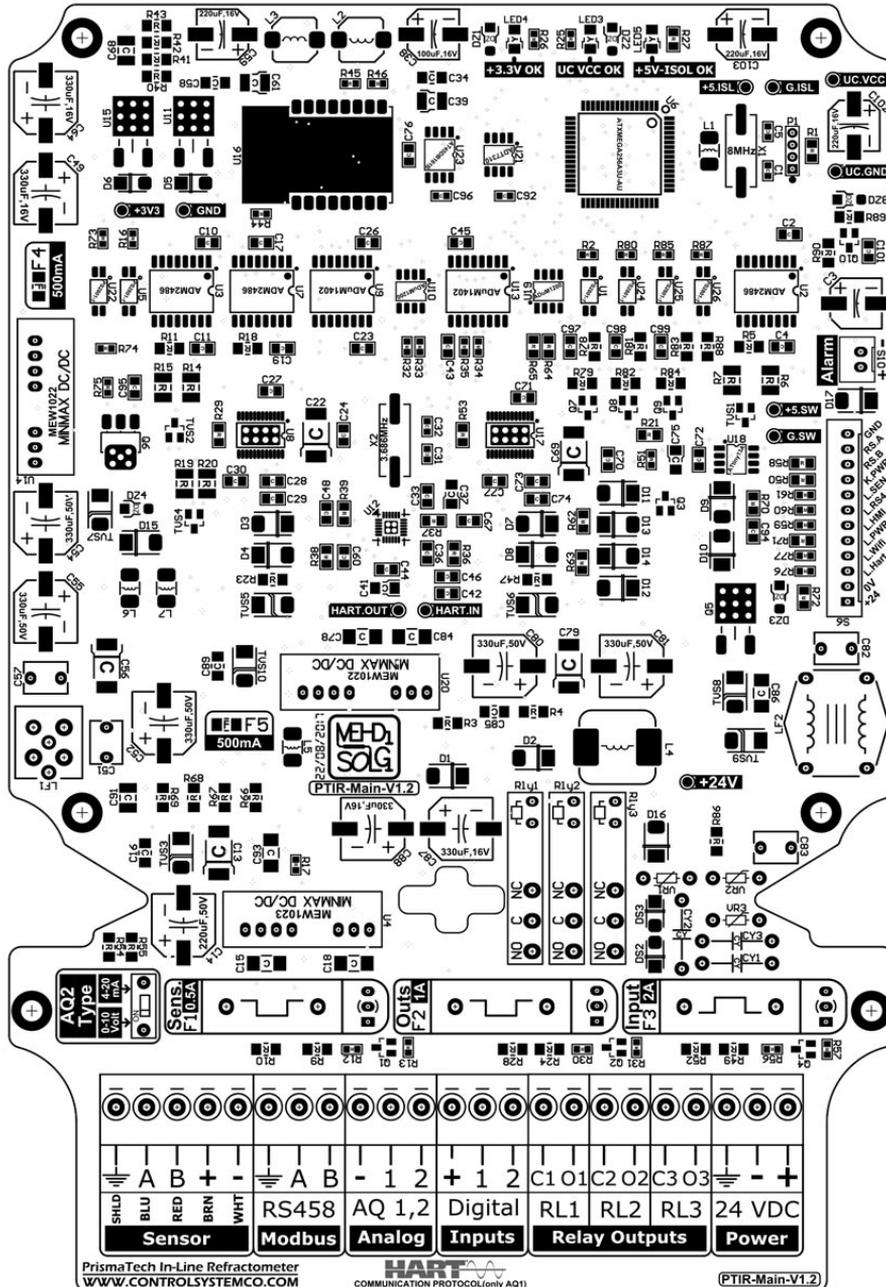
Figure 3-5 Control/Display unit Terminals
