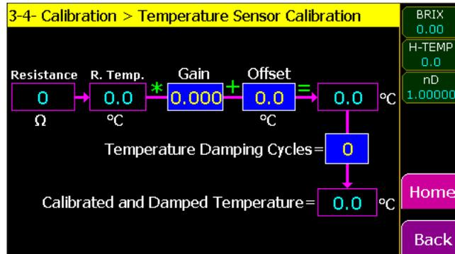
Figure 6-11 Temperature sensor Calibration
