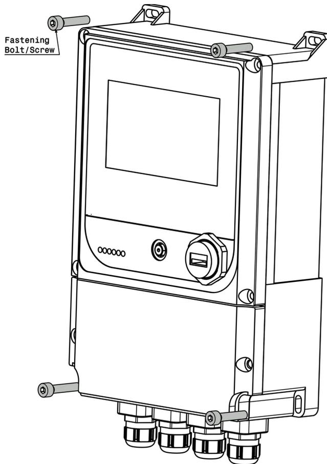
**Figure 3-3** Mounting Control/Display unit
